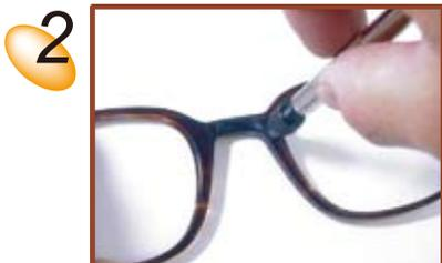
To install stainless steel pad arms insert the  $\Phi 0.7$  bit ( $\Phi 0.8$  for beta titan parts) into the drill vice so only 3.0mm of the bit is protruding. Drill the pin holes at the location designated in step 1.
