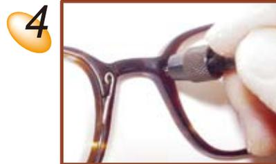
Once the basic pad arm angle has been determined and adjusted, using the grid paper again, make a mark in the center of the pad arm ring that is flush to the frame. Remove the pad arms from the holes. Insert the 1.0mm bit drill into the drill vice (extending 4.0mm) and drill a hole in the location market.
