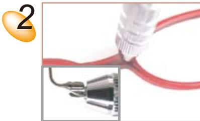
2 Using a 1.5mm drill, extend the bit by about 3mm (or the same length of the insertion point on the Titarm), and clamp it tightly. Drill a hole at the point marked on the frame in Step 1. Note: Should the frame be thinner than the protruding portion of the Titarm insert, cut the Titarm to the appropriate length.
