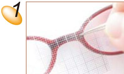
1 Detach the temples from the frame. Once you have cut off the formed nose pads, with cutters, filed down, and polished any remaining burrs, use the grid sheet to determine the insertion point of the Titarm.
