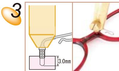
3 Insert the appropriate Titarm (L or R) into Arm Holder Tool. Taking care to make sure the angles are correct, firmly push the protrusion into the hole in the frames. (Do NOT rotate the tool while inserting the parts or it will not properly be held). Note: Once the part is fully inserted the process is complete. If you need to remove the part for reinsertion and adjustment purposes, pull the part directly out and then use a cement or bond when reinserting for subsequent trials.)
