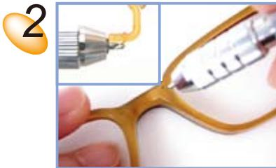
2 Using a 1.5mm drill, extend the end by about 3.5mm (or the same length of the insertion point on the Plarm2), and clamp it tightly. Drill a hole at the point marked on the frame in Step 1.
