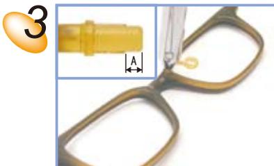
3 Place the Plarm2 into the specialized tool, and rotate the pad arm into the hole for the distance of "A" in the diagram. From that point on, take care NOT to rotate, and push the part directly into the hole.
