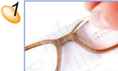
1 Detach the temples from the frame. Once you have cut off the formed nose pads, with cutters, filed down, and polished any remaining burrs, use the grid sheet to determine the insertion point of the Plarm2.
