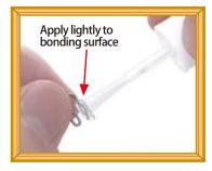
Apply the special acetate-specific bond to the bonding surface of the Pitarm. Wait 1-2 minutes.
