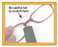
Using an acetate file, file any burrs or protrusions that may remain on the cut surface after step 1. Be careful not to file too vigorously as the shape of the frame may be changed, or difficult to remove scratches may be produced. To prevent scratches on the frame, it may be advisable to tape the surrounding areas. Buff smooth if necessary.
