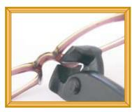
Using the special cutters, cut the plastic nose pad off the frame. Be careful not to damage or scratch the frame during this process.
