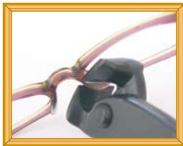
Using the special cutters, cut the plastic nose pad off the frame. Be careful not to damage or scratch the frame during this process.
